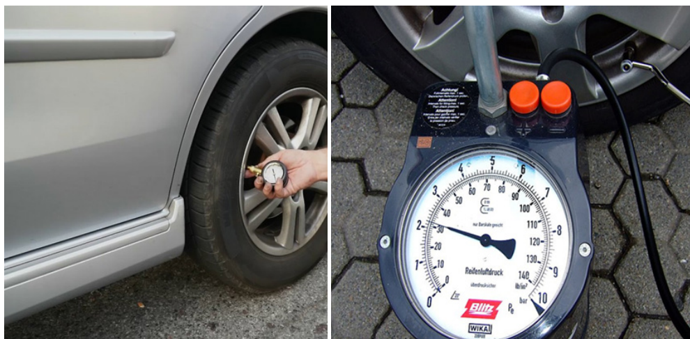
Figure 3.7: Measuring vehicle tyre pressure
